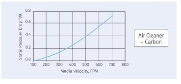
Dynamic Air Cleaners use electronic polarized-media technology to provide maximum ozone-free air cleaning. The air cleaner's efficiency increases as it loads, providing exceptionally high efficiency with air resistance much lower than passive filters.
